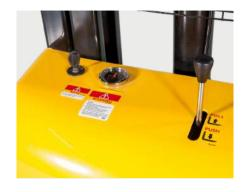
Precise lifting and lowering via hand lever. Battery cut -off key switch prevents unauthorized use.
