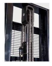
Study and reliable mast made of rolled U-profiles.
